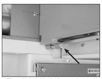
**Figure 23.** Left side of safety guard secured through welded bracket.
